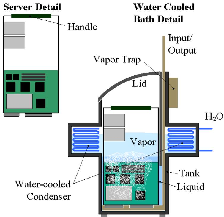
Figure 1 – Air- and water-cooled open bath immersion concepts (top). Detail of water-cooled open bath immersion concept (bottom)
