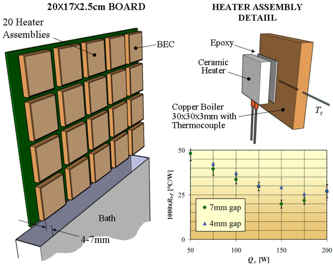
Figure 3 – Experiment (left) demonstrating the power density capabilities of immersion for a vertical PCB. Achieved 4kW per liter with only 200cc of dielectric fluid.
