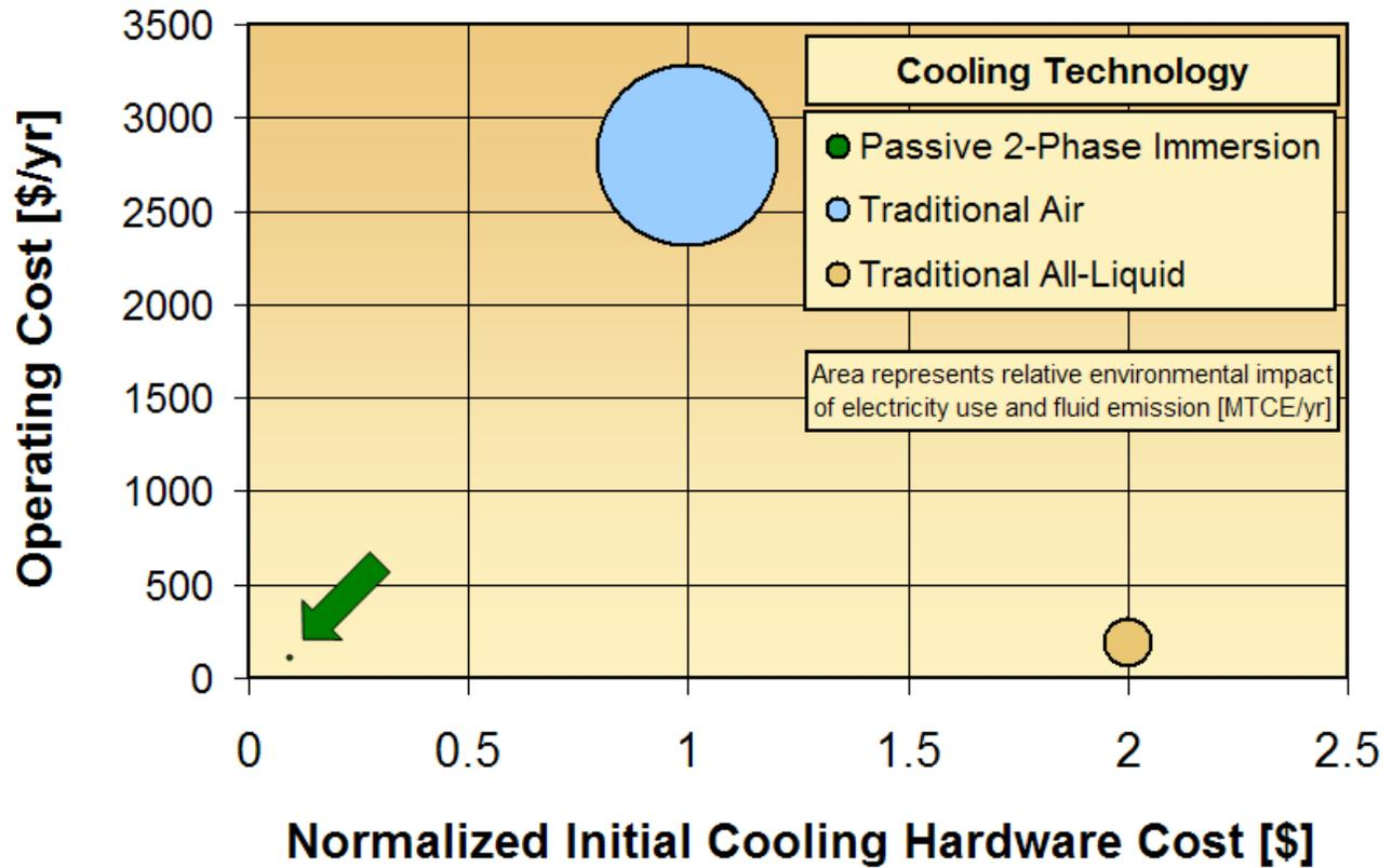
Figure 5 – Rack level initial hardware, operating and environmental, cost for modular 80kW bath versus conventional air and all-liquid solutions.
